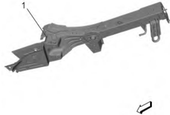
Fig. 135: Drilling Plug Weld Holes In Body Rear Rail Panel Service Part Courtesy of GENERAL MOTORS COMPANY
